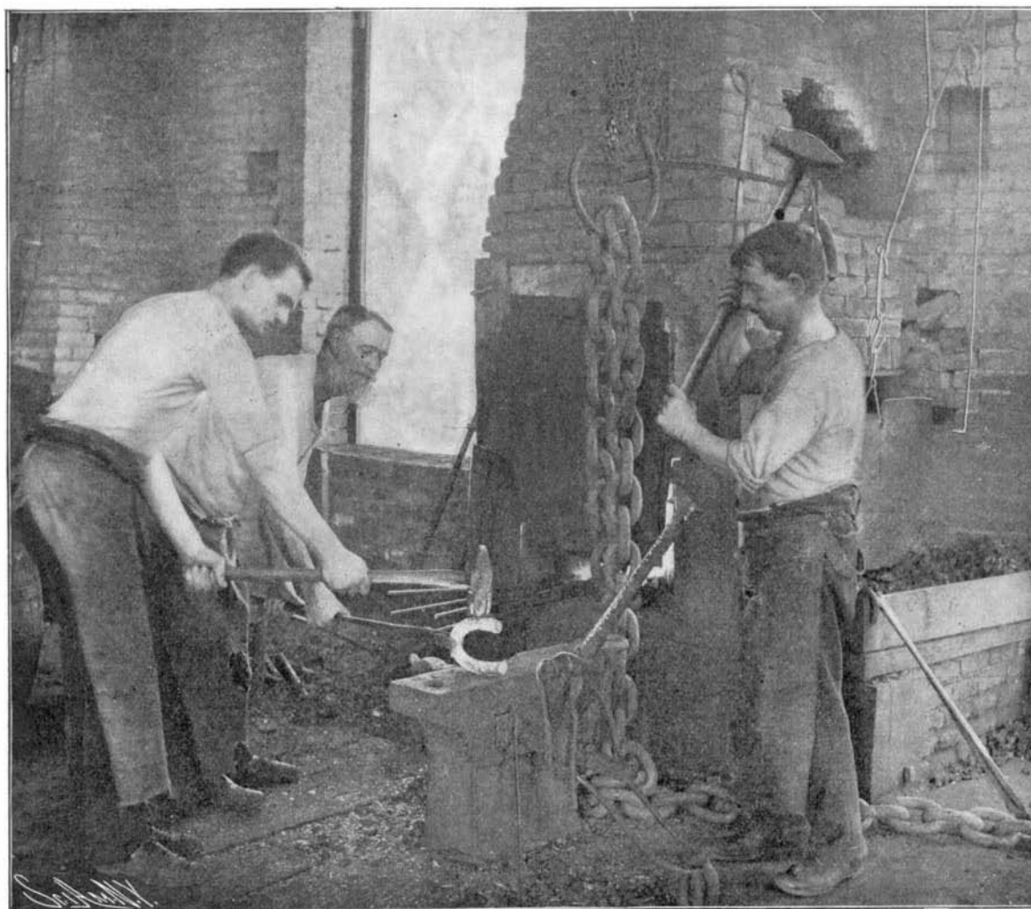
This smith and his two helpers are forging 1½-inch ship's cable at the rate of 35 links in one hour.
