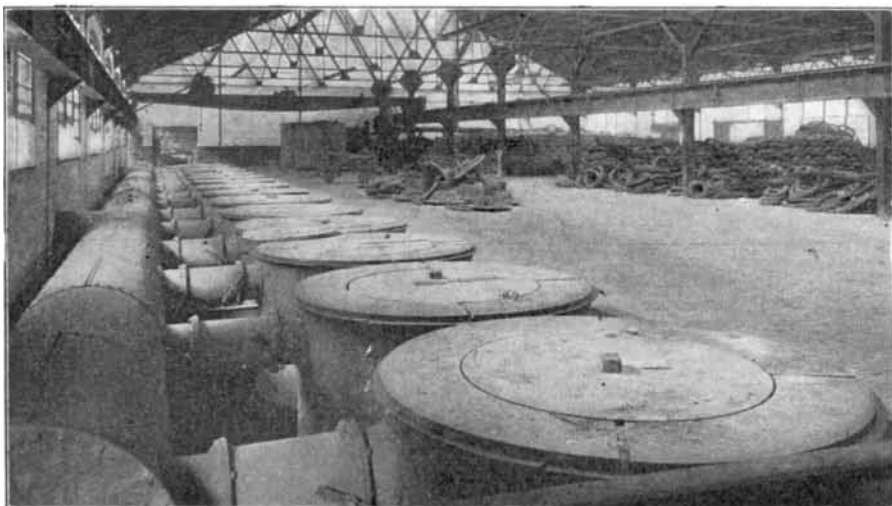
Annealing Room, Where Wire is Subjected to Steady Temperature for Several Hours to Remove Strains.
