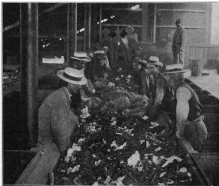
Rubbish on the Traveling Conveyer Belt. The Pickers Sort Out Over Half the Material and Sell it; the Rest is Conveyed to the Furnaces.
