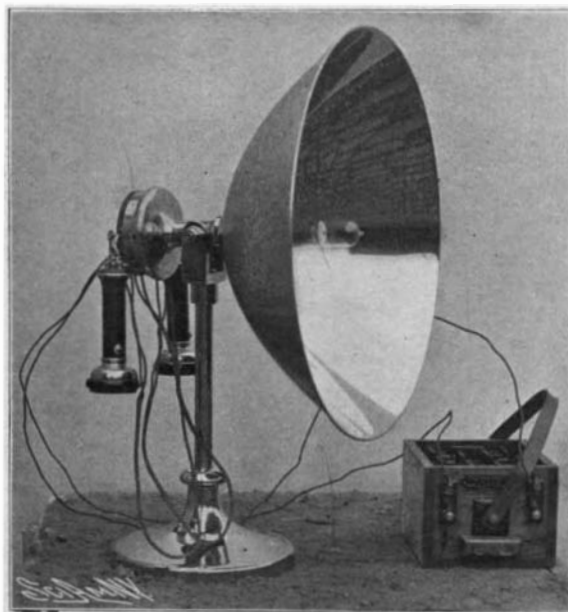
RUHMER'S CELL APPLIED TO A PARABOLIC REFLECTOR FOR OBSERVING AN ECLIPSE OF THE MOON.
