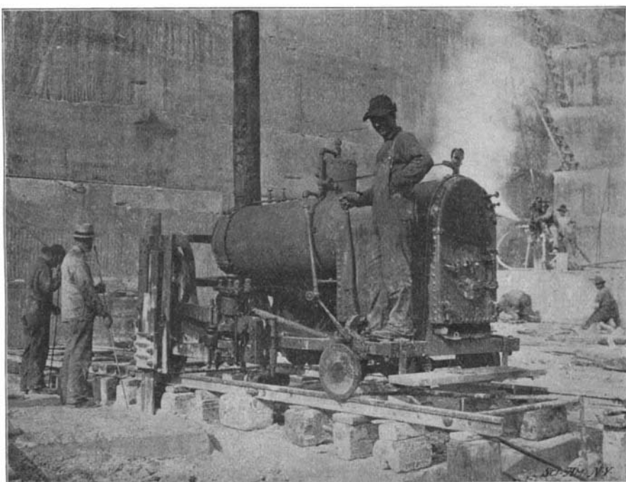
Sawing Sandstone by Machinery.
