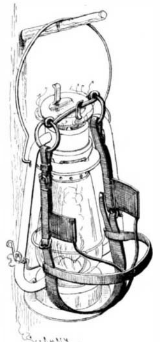
DEVICE FOR WARMING BRIDLE BITS.
