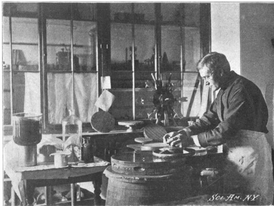
Fig. 6.—Polishing the Mirror.
