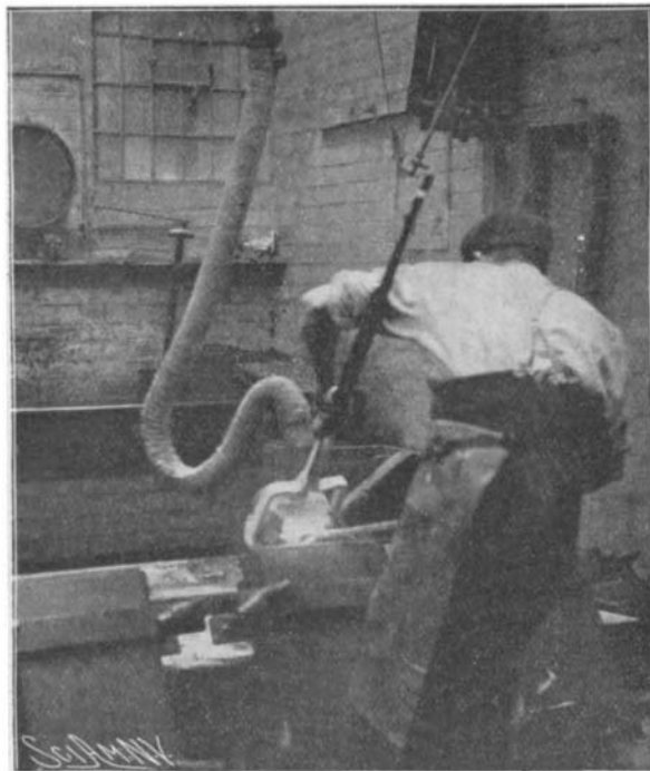
POURING BRASS BY THE LYNES METHOD Atmosphere clean; fumes escaping through flexible exhaust pipe.
