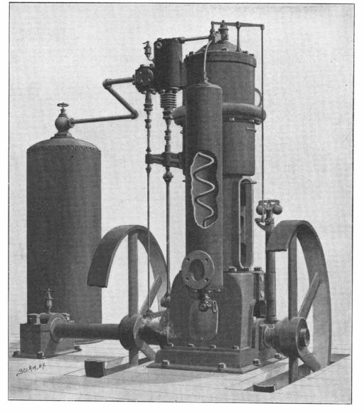
check valves,  $L^1$ ,  $L^2$ ,  $L^3$ , by which the oil is prevented from flowing back under the pressure of the upstroke of the piston A. A valve in the pipe leading from the pre-heater coil is connected with the centrifugal governor of the engine, so that the feeding of the fuel is controlled in accordance with the requirements of speed and load at any particular moment.
