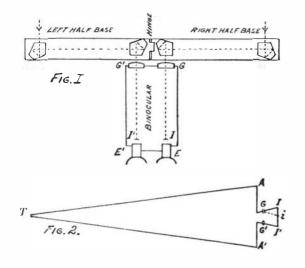
images at I' and i would be seen as one. We measure the distance I i, by the drum-head which works a micrometer screw.
