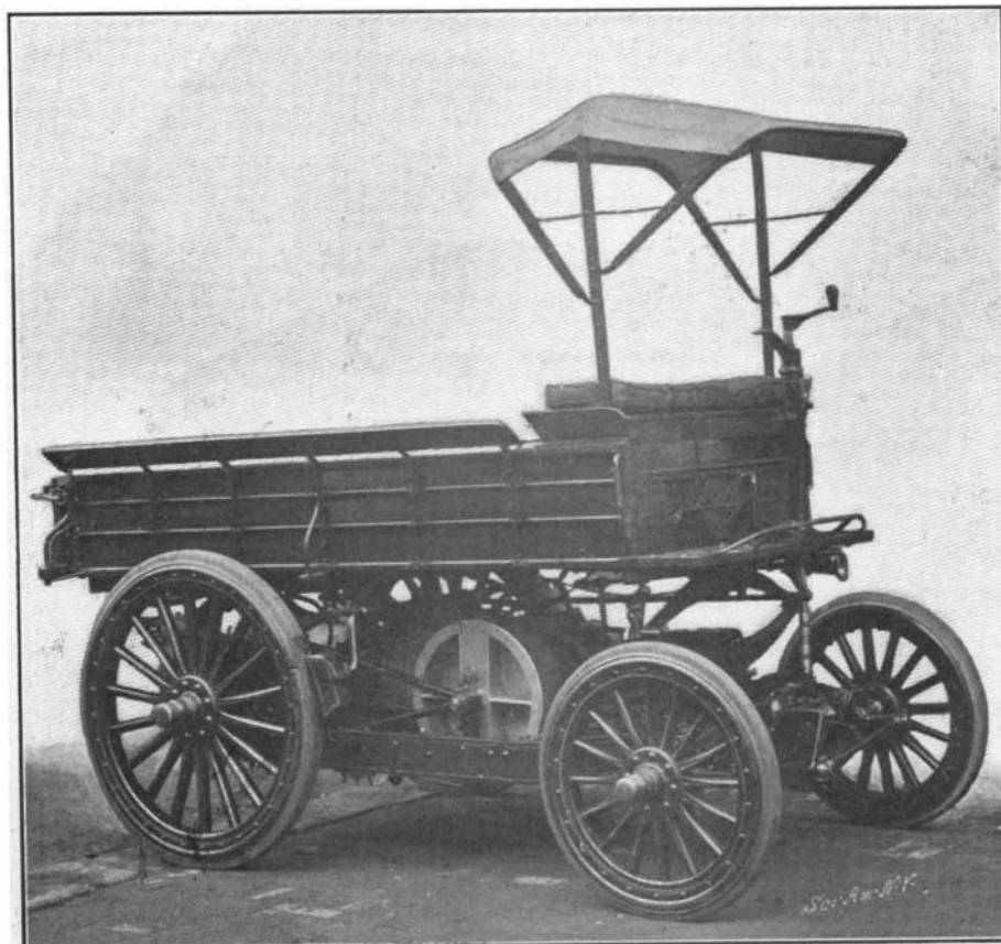
UNION GASOLINE MOTOR TRUCK, SHOWING CONNECTING RODS FROM MOTOR TO REAR AXLE.
