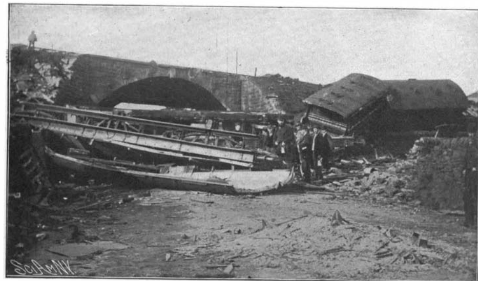
THE WRECK AT LITTLE BYTHAM, SHOWING HOW THE LIGHT ENGLISH CARS CRUMBLE TO PIECES.
