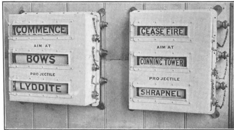
ELECTRICAL INDICATORS FOR ORDERS AND SIGNALS.
