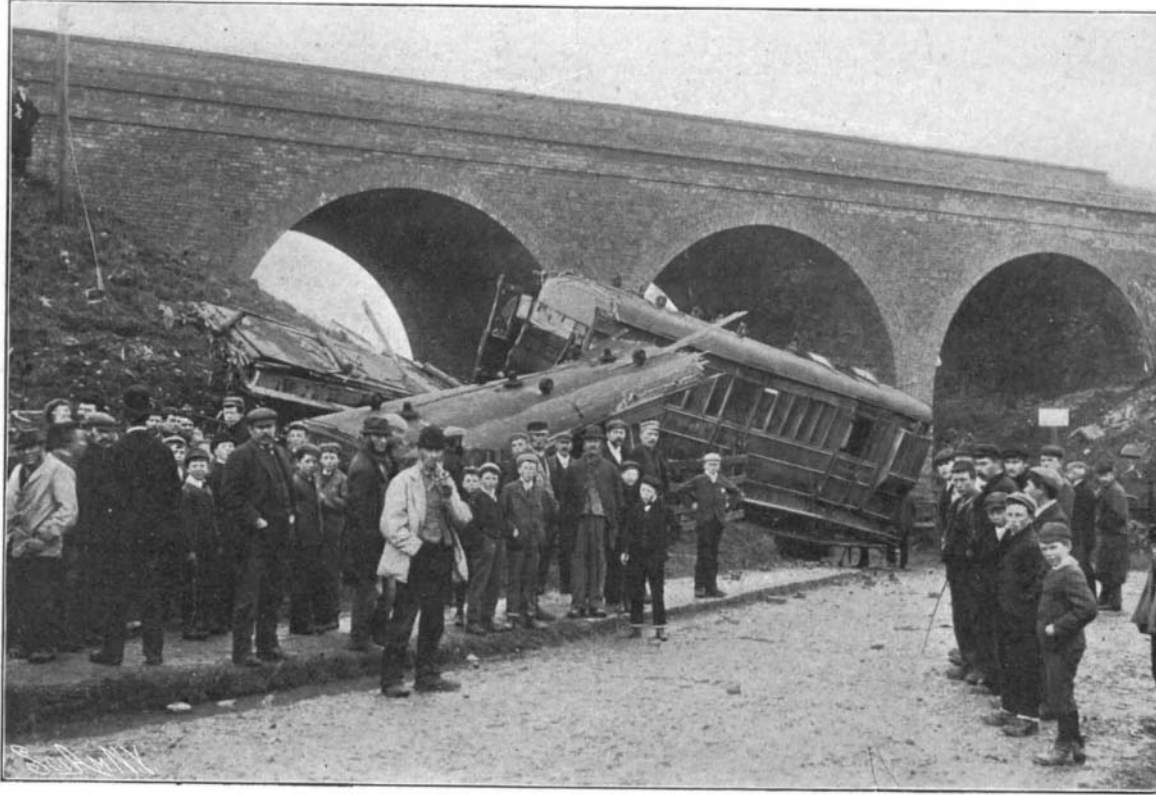
THE WRECK AT LITTLE BYTHAM. THE TRAIN LEFT THE VIADUCT BECAUSE OF THE SPREADING OF THE RAILS.
