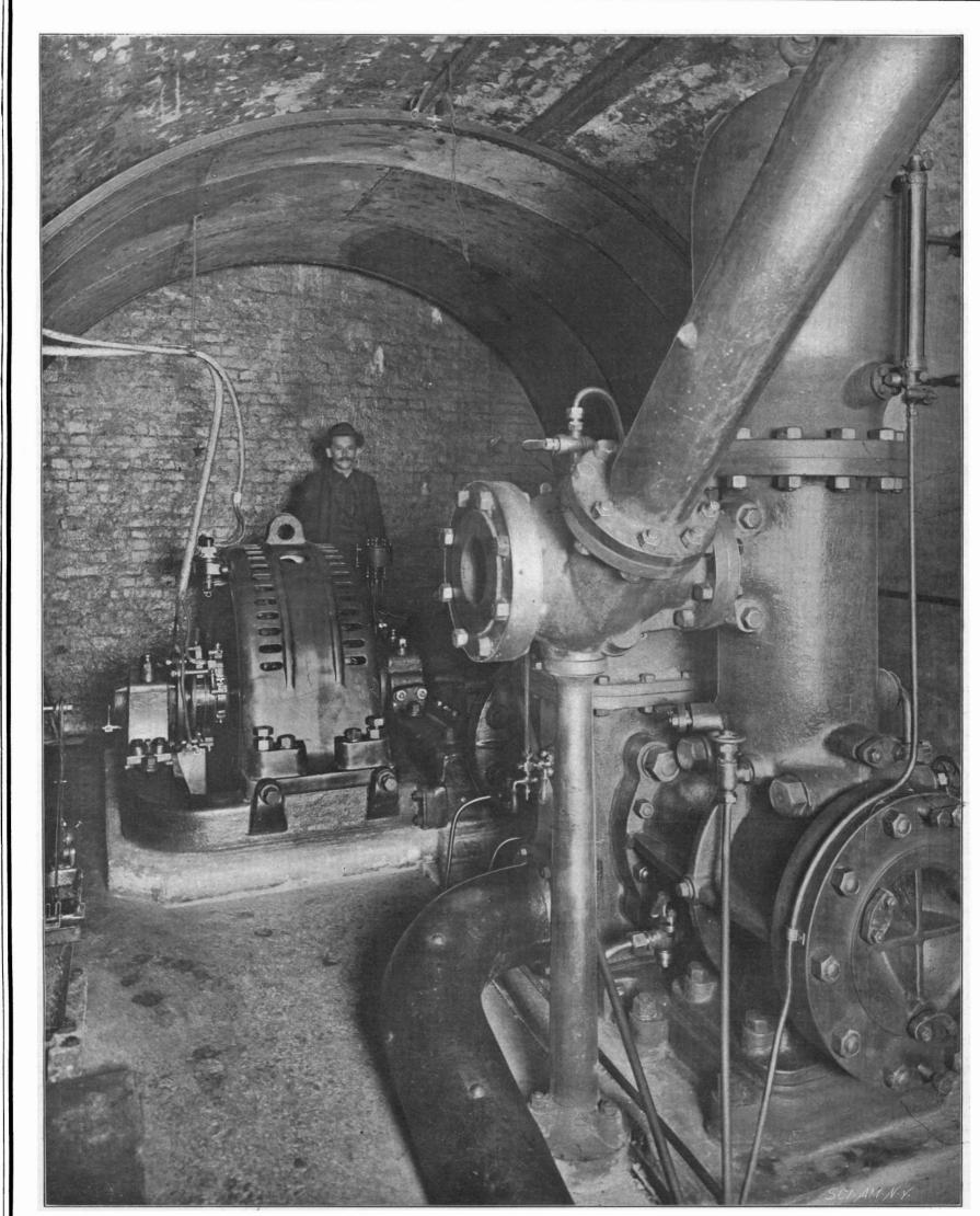
ELECTRICITY IN MODERN MINING INSTALLATIONS.—AN ALTERNATING-CURRENT MOTOR DRIVING A MINING-PUMP UNDERGROUND.—[See page 223.]
