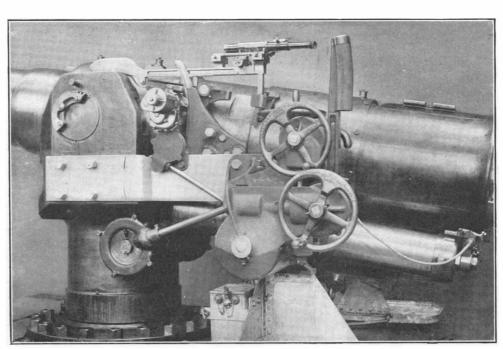
THE GRENFELL GUN-SIGHTING MECHANISM, SHOWING DIFFERENTIAL GEARS OPERATEL BY THE GUN-SETTER.
