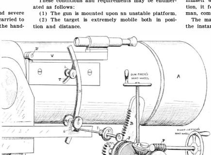
DETAILS OF THE OPERATING MECHANISM.
