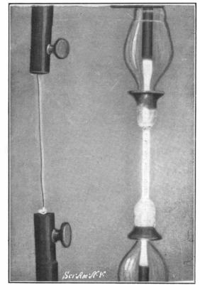
Fig. 2.—SPECTRUM TUBES MADE FROM AMOR-PHOUS SILICA.
