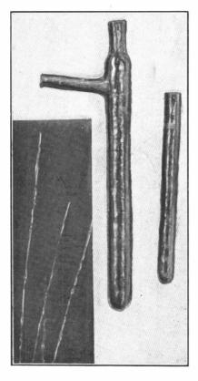
Fig. 1.—NEEDLE-LIKE PIECES OF AMORPHOUS SILICA, AND THE TUBES BUILT UP FROM THEM.
