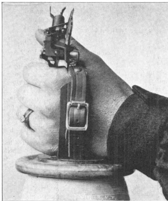
HOW THE KNOTTER IS STRAPPED TO THE LEFT HAND.
