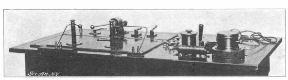
FESSENDEN COMBINED SENDING AND RECEIVING APPARATUS, REAR VIEW.
