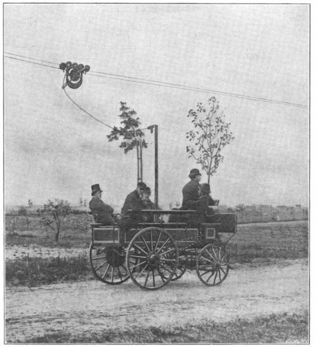
Electrical Wagon Operated by Auto-Motor Trolley.
