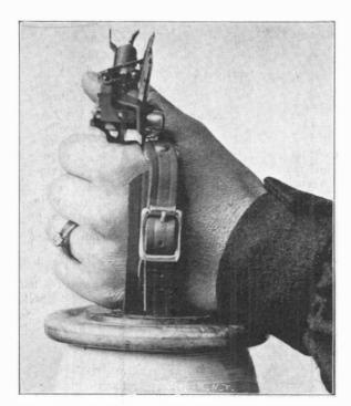
HOW THE KNOTTER IS STRAPPED TO THE LEFT HAND.
