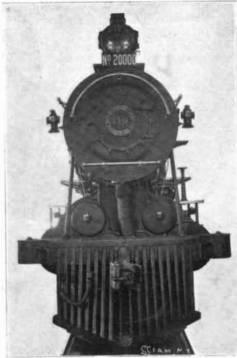
Front View of the 20,000th Baldwin Locomotive Showing Arrangement of the Four Cylinders and Two Piston Valves.
