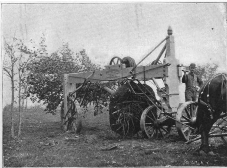
POWERFUL MACHINE FOR MOVING LARGE TREES.
