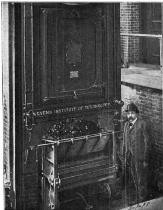
AUTOMATIC STOKER FOR SMOKE CONSUMING FURNACE.
