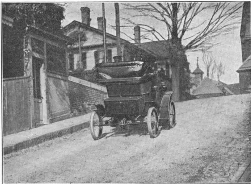
This picture was taken when car was climbing this hill of a 22% grade at 18 miles an hour
