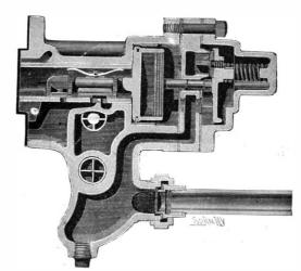
Fig 3 - THE TRIPLE VALVE.
