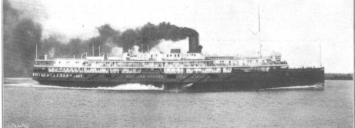
Length over all, 386 feet; breadth, 44 feet; depth, 26 feet; tonnage, 5,000; horse power, 8,000; draught, 16 feet 8 inches; speed, 22 miles an hour.
