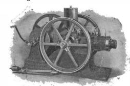
THE MIETZ & WEISS DIRECT COUPLED GENERATOR AND KEROSENE ENGINE
