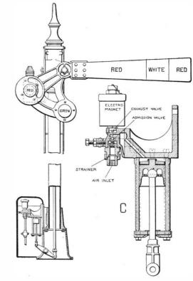
Fig. 3.—Details of Electro-Pne matic Semaphore.
