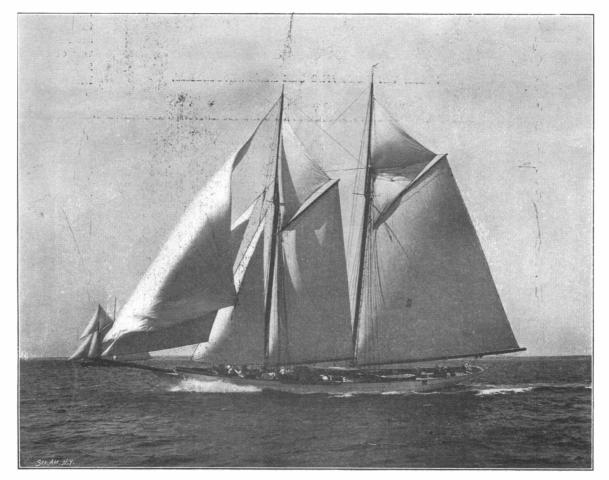
Length over all, 131 feet; waterline length, 110 feet; beam, 26 feet; depth, 19 feet; draft, 14 feet. Compound engine: High pressure, 9 inches; low pressure, 19 inches; stroke, 14 inches.
