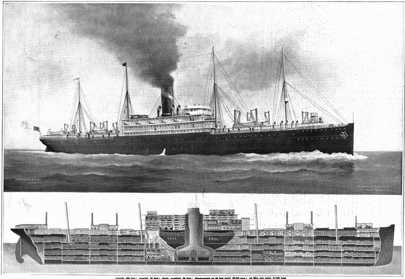
Length, 680 feet; breadth, 73 feet; depth, monided, 56 feet; displacement on 83 feet draft, 38,000 tons; on 36½ feet draft, 37,000 tons.
