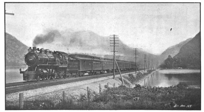
Albany to Spuyten Duyvil, 131.7 miles, was run in 131 minutes. Excluding the time lost in eight slowdowns, the average running speed was 68 miles per hour; weight of train, 352.6 tons; of engine, 144 tons.
