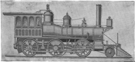
Fig. 8.—" Mogul" Engine. 1863 New Jersey R.R. & Transportation Co.
