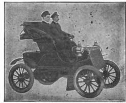
1903 Model is 50 per cent. stronger and more durable in every detail than the 1902 Model. Wood wheels, 3% inch. clincher tires, longer wheel base, larger and more powerful air-cooled engine, larger and more comfortable folding front seat, easily carrying two adults. Price. \$1200.
