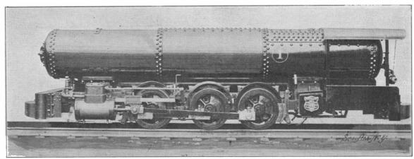
Locomotive Driven by Compressed Air.
