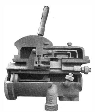
Fig. 2.—THE ENGINEER'S VALVE.
