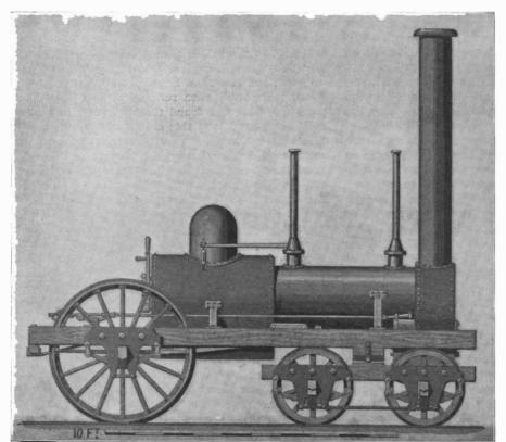
Fig. 6.—The "Experiment." 1832. First Engine With a Leading Truck.
