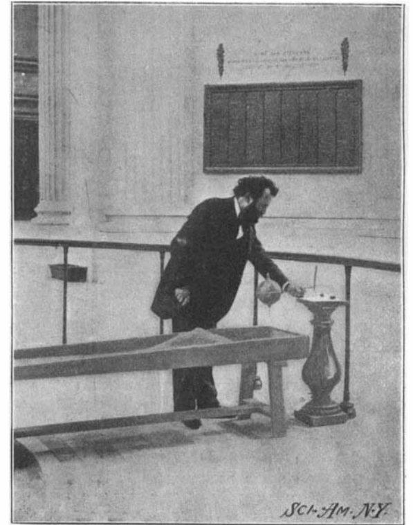
FLAMMARION STARTING THE PENDULUM BY BURNING THE SILK STRING WHICH HOLDS IT.
