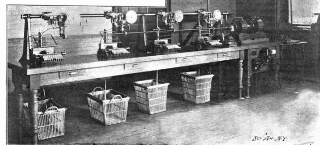
A Group of Keyboards. Main Line Relay and Transmitter to the Right.
