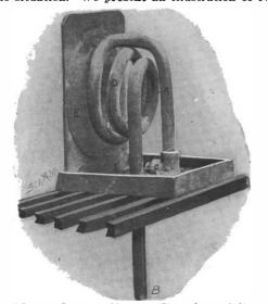
Detail of Range Burner, Showing Vaporizing Coil and Reflector Lamp.
