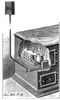
Range Oil Burner in Which the Oil is Fed by Gravity.
