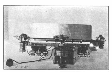
Printer, Showing Combination Commutator and Distributing Relays.
