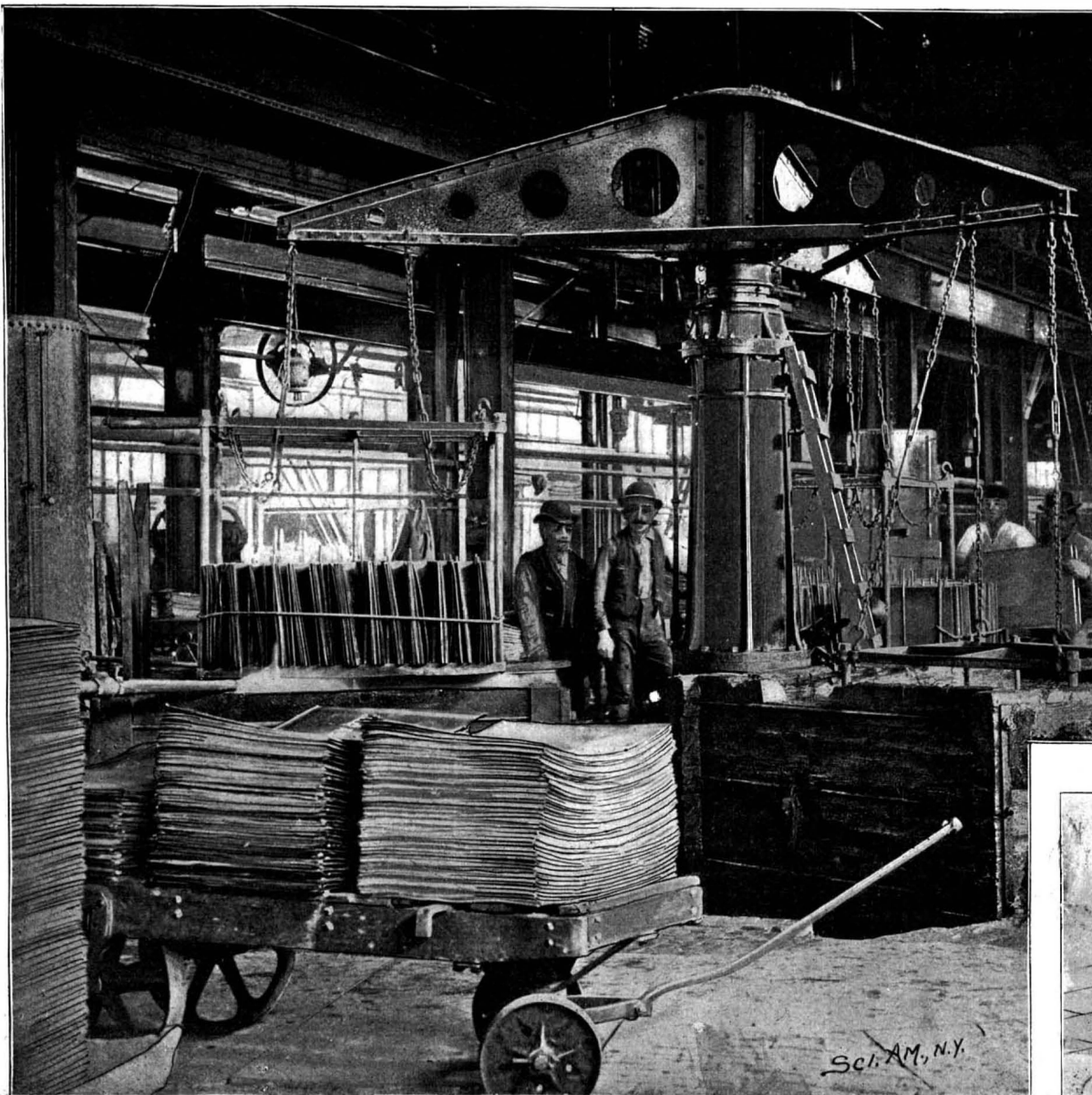
The Pickling Machines for Cleaning Plates Preparatory to Tinning.
