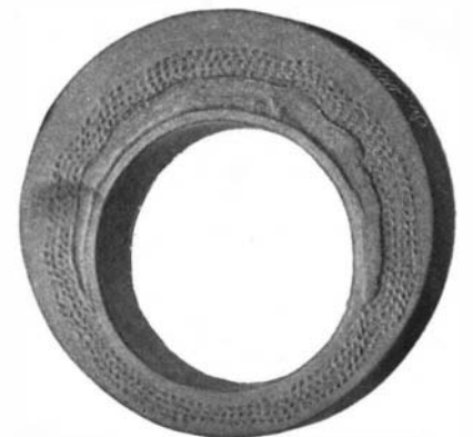
Fig. 7.—Non Puncturable Tire with Layer of Fiber.
