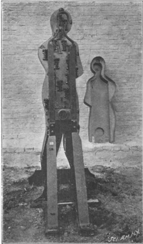
BACK OF THE DUMMY TARGET WITH COVER REMOVED.
