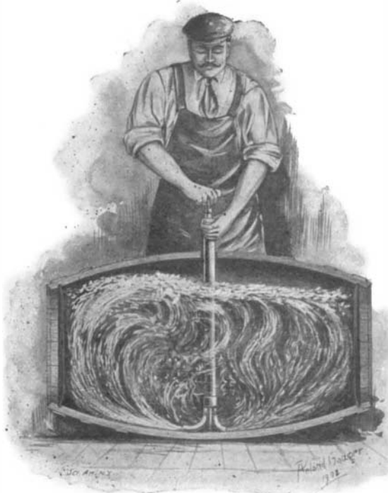
MIXING PUMP IN OPERATION.
