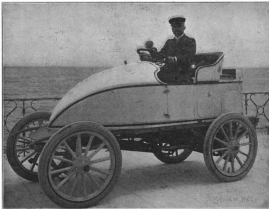
SERPOLLET'S RECORD-BREAKING STEAM RACER.
