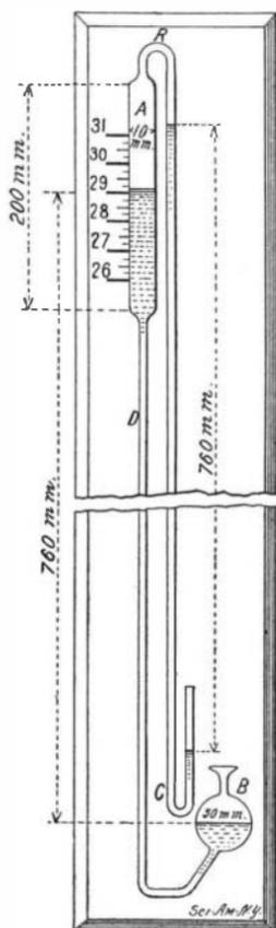
tube is then bent as shown, and to the end of the length, D, is sealed the bulb, B, whose diameter is about 5 centimeters. In bending the tube care must be taken that the dimensions given on the drawing are carefully adhered to. The whole tube must then be carefully cleaned with nitric acid, and is then washed in succession with distilled water, alcohol, ether, and dry air. It is then attached to a suitable frame, and is ready to be filled with mercury.
