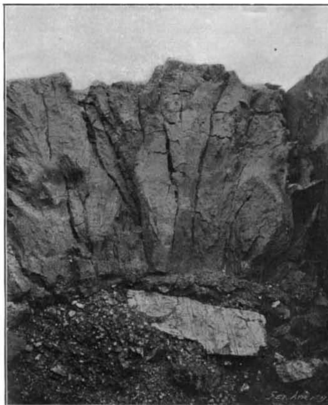
Partly Coked Contents of a Coke Oven.
