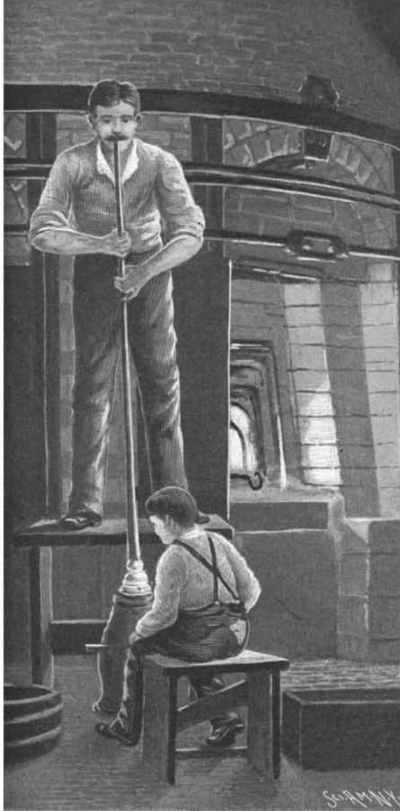
Forming the Chimney in the Mold.
