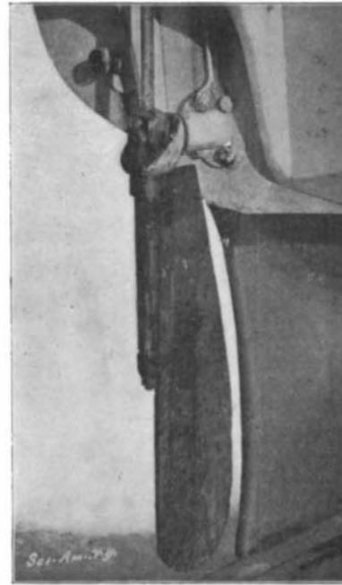
PROPELLER DRIVING ASTERN.
