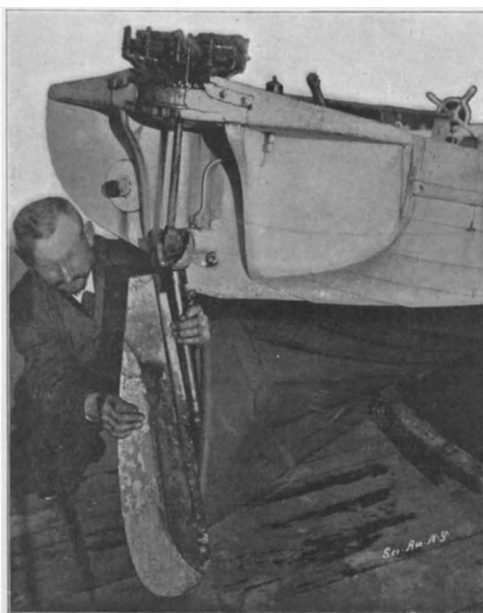
VOGT'S PENDULUM PROPELLER, SHOWING BALL-AND-SOCKET JOINT AND STEERING MECHANISM.
