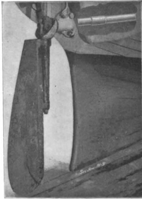
PENDULUM PROPELLER DRIVING FORWARD, SHOWING SHAFT.
