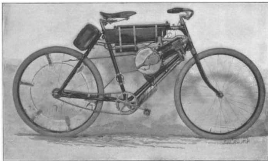
The Mitchell Motor Bicycle (2 H. P.) with Flexible Rawhide Belt.
