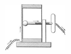
current follows the path indicated by the arrows, passing from the metallic diaphragm to the metallic sphere in contact with the same. The screw serves to adjust the contact between the diaphragm and the sphere.
