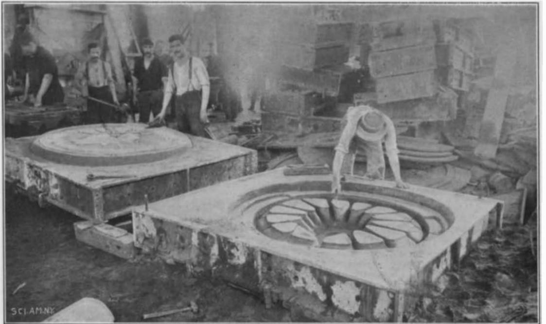
Finishing Mould for Locomotive Driving Wheel.
