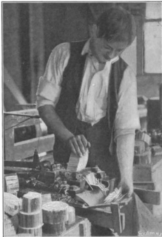
The splints are cut by a reciprocating knife from the two-inch blocks of cordwood.
