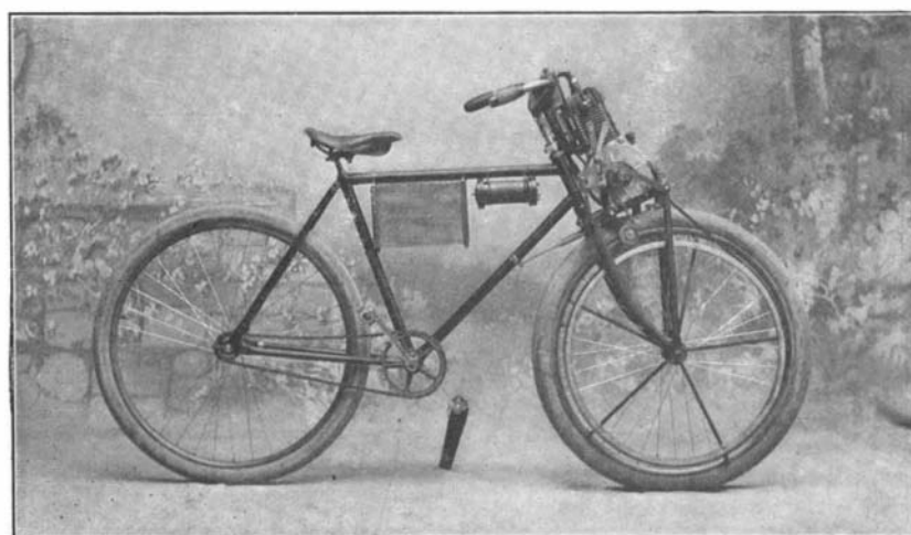
MOTOR-CYCLE WITH MOTOR CARRIED ON FRONT FORKS AND DRIVING FRONT WHEEL.
