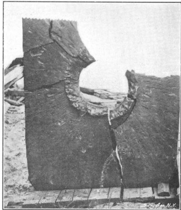
Armor-plate 5 3/4 inches thick, After Penetration by 12-inch Shell Carrying 70 Pounds of Maximite.
