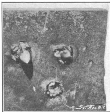
3-Inch Plate with 6-Pounder Shells Embedded Without Exploding.
