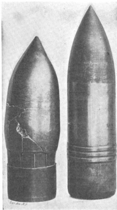
A 6-Pounder Armor-piercing Shell, Filled with Maximite Before and After Firing Through a 3-Inch Armorplate. The Shell Upset and Rebounded Without Exploding.
