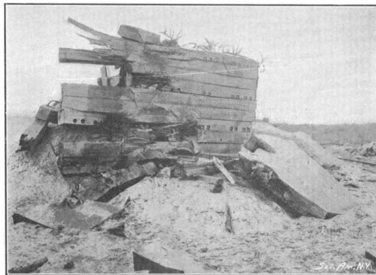
Wreck of 12-inch Plate After Penetration and Explosion of 12-inch Shell.
