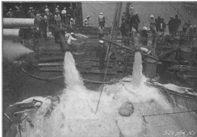
FORWARD DECK OF THE "OREGON," SHOWING TWO 10-INCH STREAMS DISCHARGED FROM THE FLOODED COMPARTMENTS.
