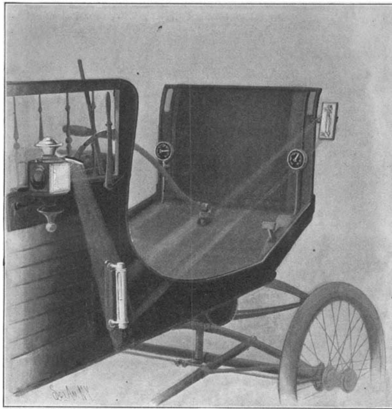
ILLUMINATING THE WATER-GLASS AND PRESSURE-GAGES OF THE LOCOMOBILE.
