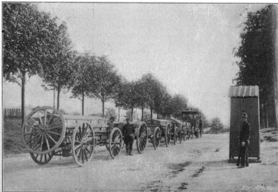
AMMUNITION WAGONS ON 8 PER CENT GRADE—TOTAL WEIGHT, 18 TONS.
