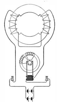
Fig. 2.—ELECTRICAL CONNECTIONS OF MOTOR.
