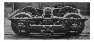
A Motor Truck, Showing Third-Rail Contact Shoe.
