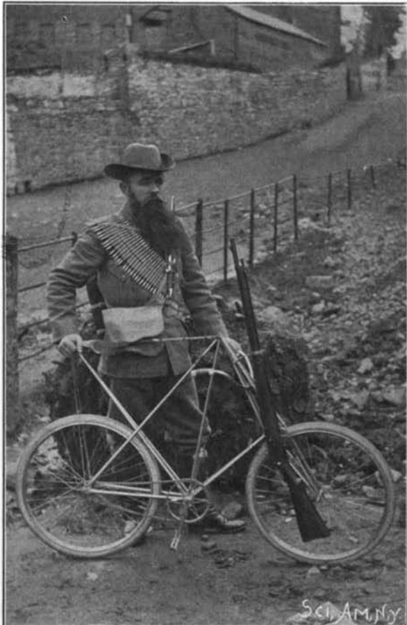
FOLDING BICYCLE, WITH RIFLE ATTACHED. WEIGHT, 15 POUNDS.
