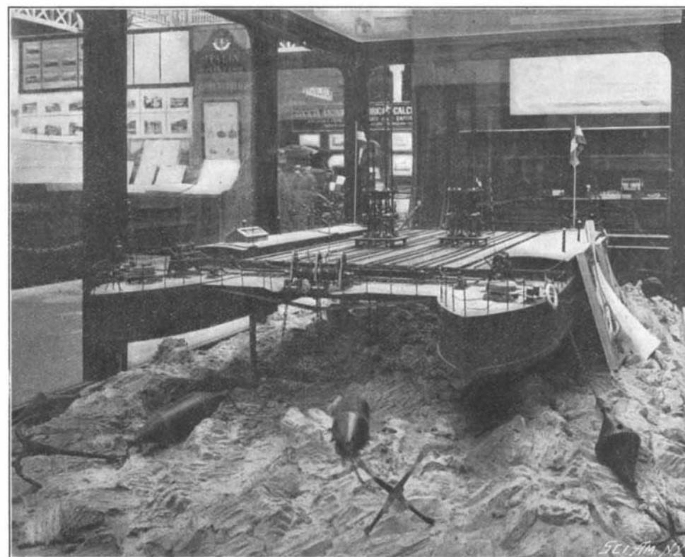
MODEL OF SOUNDING BOAT, USED ON THE DANUBE.
