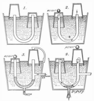
DIAGRAM ILLUSTRATING PRINCIPLES OF OPERATING THE PNEUMATIC LOCKS.
