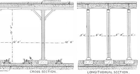
10.—CROSS SECTION AND LONGITUDINAL SECTION, SHOWING STEEL-AND-CONCRETE CONSTRUCTION.
