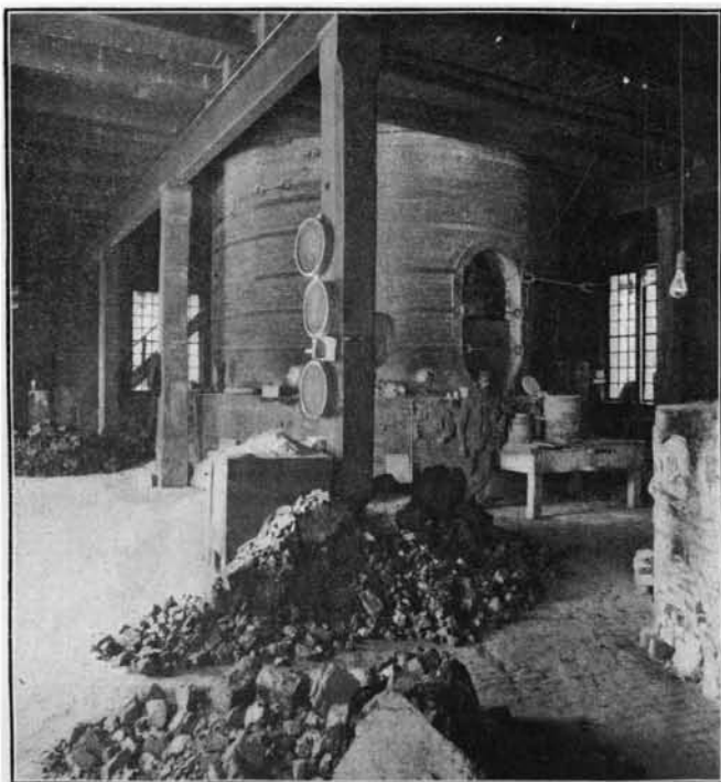
Kiln in Which the Wheels are Baked.
