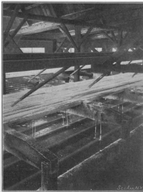
TOP VIEW OF A GRAINER, SHOWING THE BRINE, RUNWAY, AND AGITATING PADDLES.
