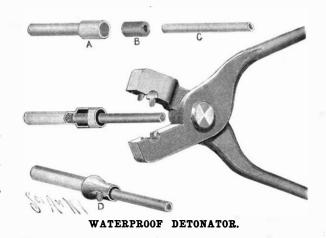
the fuse, C, and gasket, B, have been placed in position, the thim ble is crimped so that the gasket is firmly compressed around the fuse, C (Fig. 3). Displacement of the parts is thereby rendered impossible. The cap is firmly held on the fuse; and the connection between the cap and fuse rendered absolutely waterproof.
