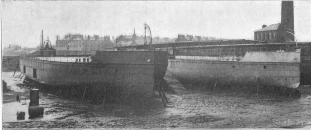
STEEL BARGES FOR SERVICE ON THE AMUR RIVER—TRANS-SIBERIAN RAILROAD. Length, 210 feet; beam, 35 feet; depth, 9 feet; Capacity, 400 tons on draught of 3 feet 6 inches.
