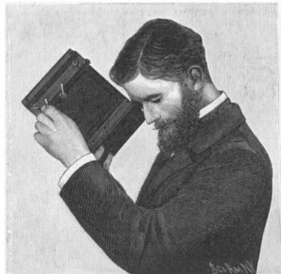
Fig. 2.—USING THE CAMERA FOR VIEWING THE POSITIVE IN COLORS.
